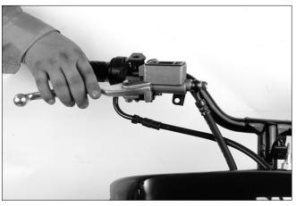
If the brake bleeder is not used, do the following. First, fill the brake fluid up to the upper limit line. Connect the hose to the bleeder valve to receive brake fluid.
